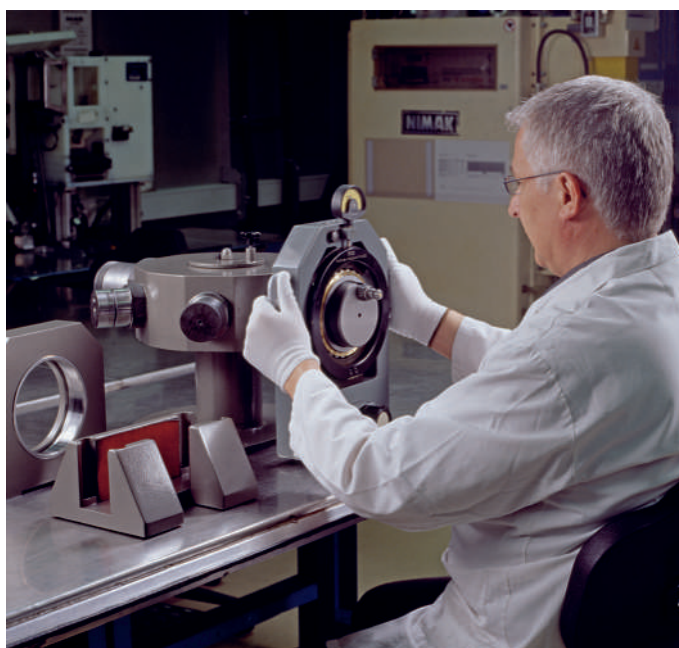
34 Positioning the enveloping circle gauge
